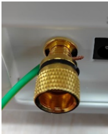
Grounding method 1: insert the grounding cable through the hole on the grounding knob.
