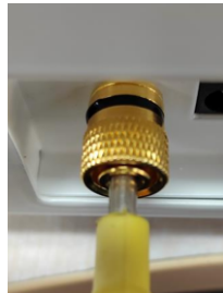
Grounding method 2: Insert an 4mm elastic rubber plug into the grounding knob.
