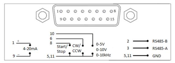
Pin 1: External speed control signal (4-20mA) input. Connected to 4-20mA signal +. The speed is in linear correlation with signal.
