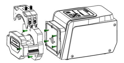
Mount the mounting plate on the drive unit through four screws M4X10. Remove the tubing and the pump head cartridges. Insert the tang of the pump head shaft into the slot of the black rubber coupling. Press the pump head firmly against the pump drive. Turn the pump head to align the mounting holes on the pump head with the mounting holes on the pump drive. Insert the 3 screws M4X16, then tighten them.
