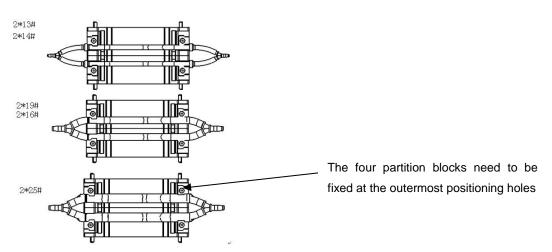
Put the compression block with tubing fitting assembly back to the pump head, and lock the levers.
