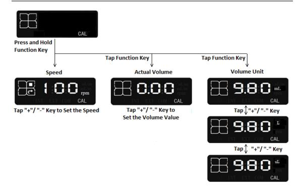
Flow rate calibration procedure:
