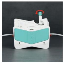
Turn the knob clockwise, the position of the knob becomes lower, the pressure tubing gap is reduced accordingly. And if the pump head tubing outlet pressure increases, the flow rate becomes lower.
