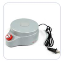
Magnetic stirrer is an instrument for liquid mixing, mainly used for liquid reagent configuration, stirring low viscosity liquid or solid-liquid mixture; MS-150 magnetic stirrer has a large stirring volume, stable rotor rotation, no jumping sub, and its shell is molded by flame retardant reinforced plastic as a whole, fully enclosed waterproof and rustproof.
