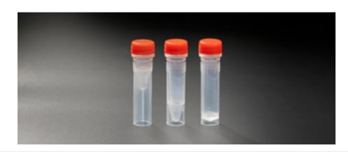
Servicebio screw cap tubes, which are with lids and without rubber rings, can be used for various biochemical reagents or sample storage and low-temperature storage, the standing round bottom design is more conducive to the concentration, recovery, and placement of samples.
