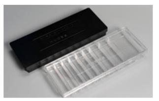
The Servicebio Antibody Incubation box is designed specifically for WB, with a transfer film placed in each box for subsequent immune incubation. It can be used with Servicebio multi-function shaker DS-3D100. The large tray can support multi-layer stacking of incubator boxes and batch incubation of multiple films at the same time.
